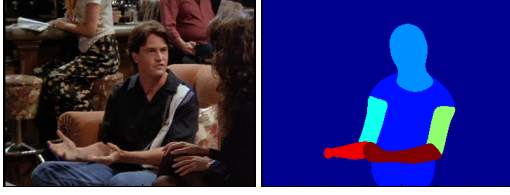
Figure 2. DS puppet layer. (1) Frame; (2) Corresponding puppet layer with parts ordered by fixed order. The warmer the color, the closer to the camera.
